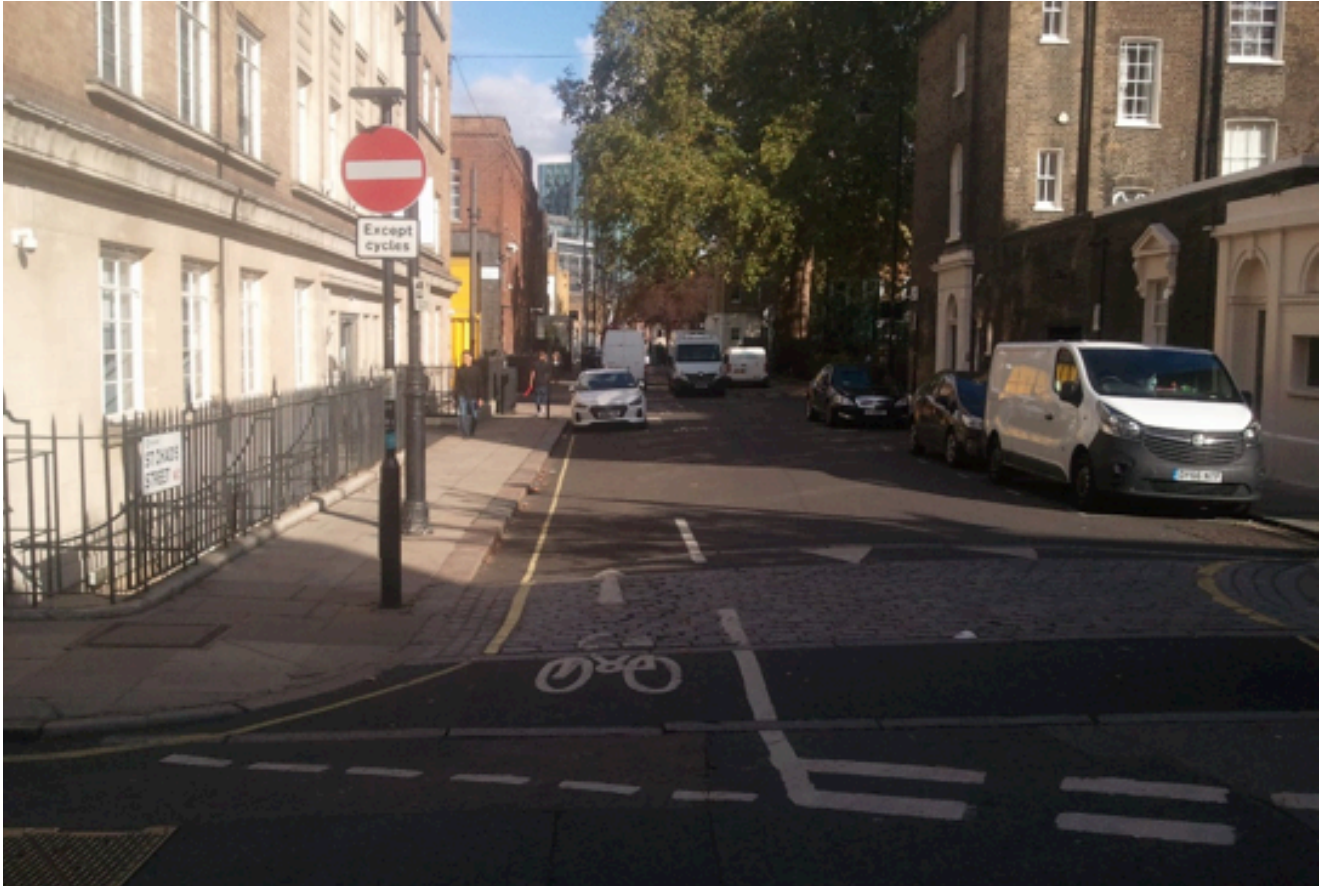
Figure C2: Exempting cycles through a no-entry for vehicles, delivering improved connectivity for cyclists
